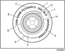
A. Tire Manufacturer The name of the tire manufacturer is shown here. B. Tire Name/Model
